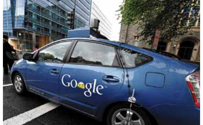
Laws in the United States require that during the testing, a driver be seated in the car even though the car is driving itself. Note the equipment fixed to the roof – this collects information on the road around.
